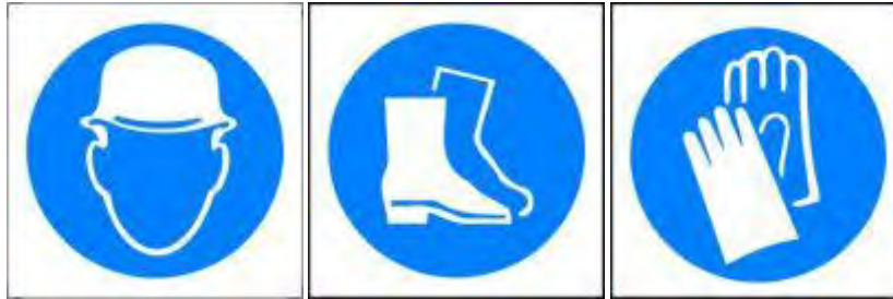
Figure 9 Signs concerning the mandatory use of protective equipment
